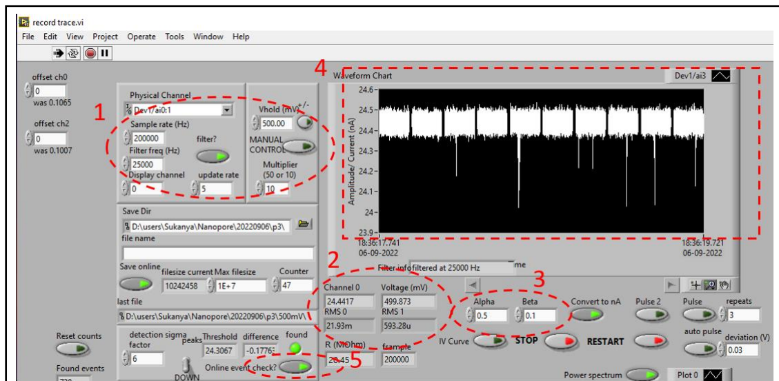
Figure 2.11: LabVIEW interface for recording current measurements.
