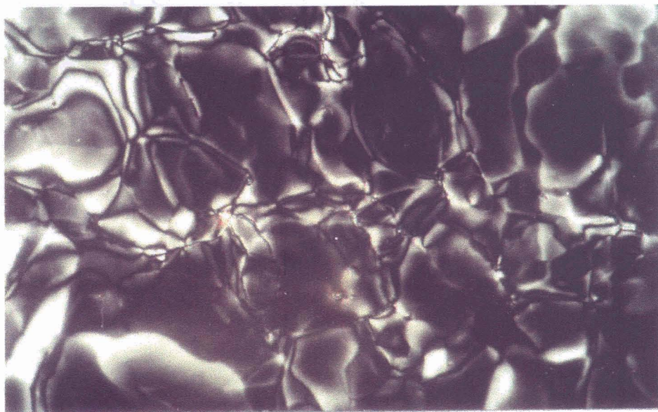
Plate 2.5 : Photomicrograph of compound 2 showing \text{Sm C}^*_{\gamma} phase (homeotropically aligned) at 116.7^{\circ}\text{C} .
