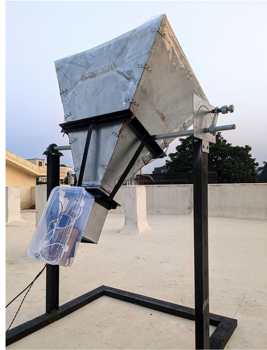
Figure 1. Pyramidal horn radio telescope. The horn antenna is mounted on a support stand with an elevation locking mechanism. The signal processing electronics are housed in the plastic box, with AC power and USB cables connected.
