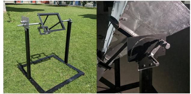
Figure 5. Support structure used to mount and orient the feedhorn assembly. Left: the support stand without the feedhorn, showing the square base, the vertical supports, and the horizontal axle that allows rotation in the elevation plane. Right: the elevation locking mechanism, consisting of a threaded locking screw engaging with a perforated steel plate fixed to one of the vertical supports. The array of holes in the plate, spaced at 5° intervals along a semicircular arc, allows the feedhorn elevation to be held securely at discrete angles during observations.
