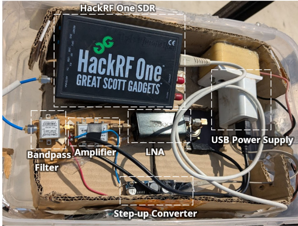
Figure 7. Image of the RF signal chain, in a plastic watertight box next to the waveguide, into which the right-angle SMA connector extends. The two amplifiers are seen connected to the dual-port USB phone charger which powers them. The digital signal (white cable) from the HackRF One and the AC power (red and black wires) extend away from the frontend box to a secure room 10 m away, where the Raspberry Pi is.
