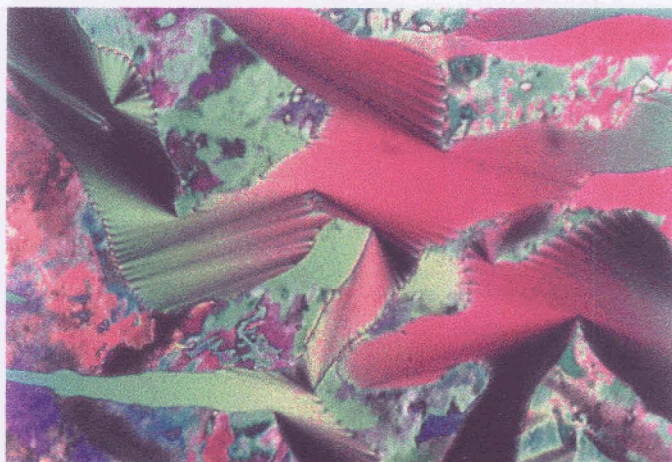
Fig.2.19. The optical photomicrograph showing B 6 phase developing from a nematic phase, compound 2.E.2, 190.5°C.
