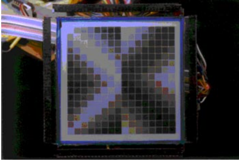
Figure 8. Photograph of a 16 \times 16 matrix LCD using successive approximation technique to display eight gray shades.
