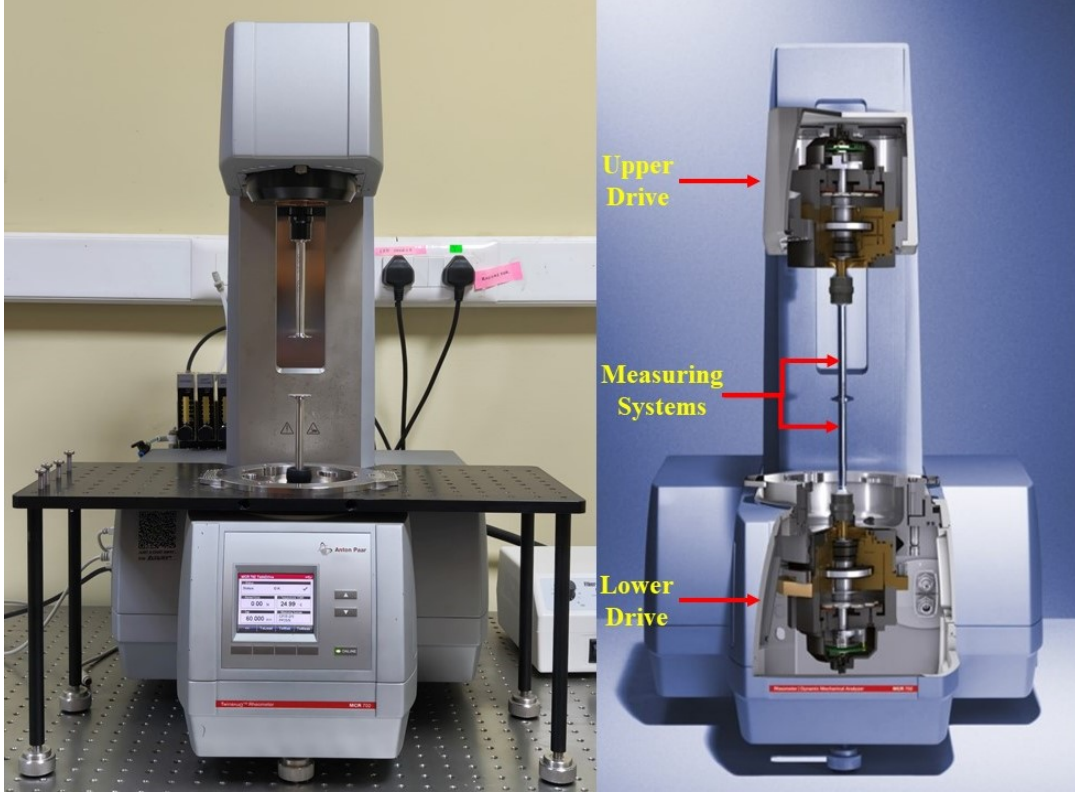
Figure 2.1: Image of Twin drive MCR 702 rheometer used for this thesis work (left) and the corresponding schematics showing the simultaneous arrangement of two fully functional rheometer drives in a single instrument (right) (figure adapted from [3]).
