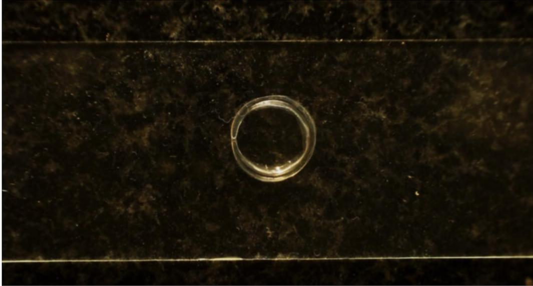
*Figure A7.5 AFM Sample Fluid Cell: A 100  $\mu$ L circular fluid cell made of silicone glue on a glass slide for AFM sample preparation.*
