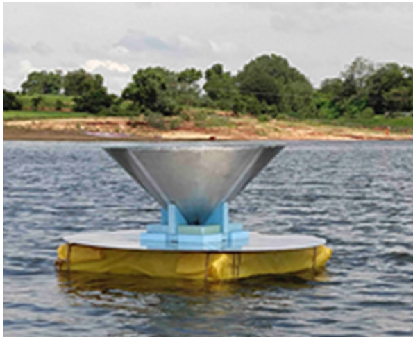
Figure 1. (Left) Photograph of the cone-disc antenna with raft deployed on the water surface of a lake. Figure 2. (Right) Measured total efficiency of the antenna. Also shown are efficiencies expected from WIPL-D and FEKO electromagnetic modelling. The total efficiency measured on real earth is also shown for comparison.
