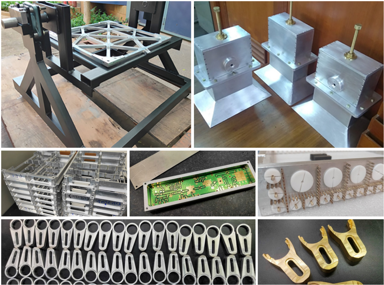
Left panel from top: trolley with rotary base and an aluminium tray to hold electronics for the X-ray polarimeter (POLIX) being built at RRI and Teflon anode bush for use in X-ray lab. Right panel from top: Pyramidal horn antenna, electronic chassis fabricated for EEG and brass clamp for holding optical posts. Bottom panel: clamps for holding optical posts.
