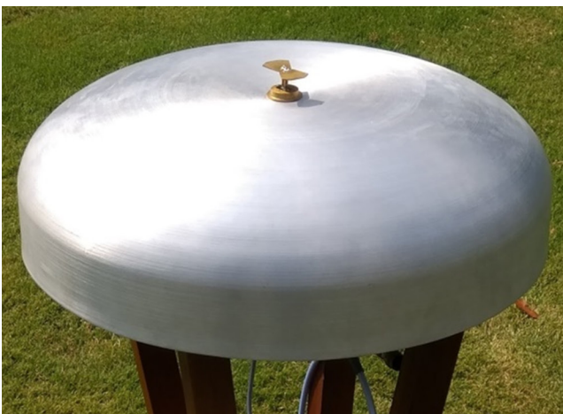
Figure 7. (Left) Log-spiral reflector based octave bandwidth frequency independent dipole antenna Figure 8. (Right) Spectrally smooth return loss characteristics of the antenna.
