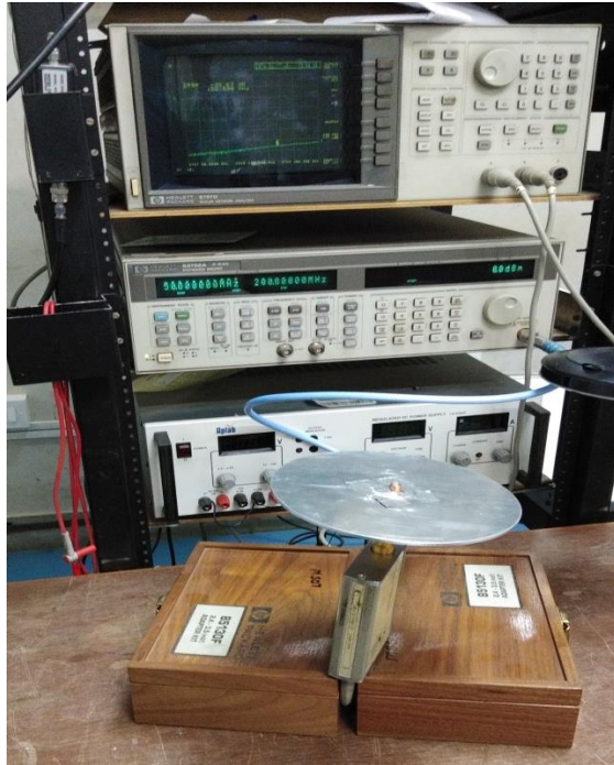
Fig. 4. Experimental setup for characterizing the load designed for calibrating the receiver at the antenna port.
