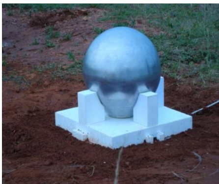
Fig.13. Prototype of the spherical monopole antenna. Styrofoam is used to support the antenna structure
