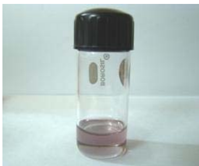
Figure 2. Shows the photograph of decanethiol stabilized gold nanoparticles dispersion in toluene.
