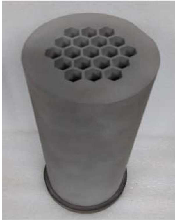
Fig. 6.11 Small collimator used for the calibration of modulation pattern produced by an off-axis source due to the spin of satellite. Image Credit: Rishin P.V.
