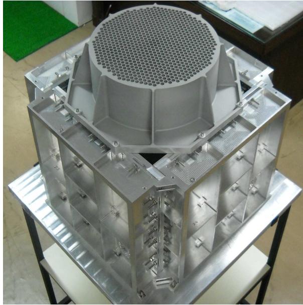
Fig. 2.6 Aerial view of POLIX assembly in the lab. A collimator is seen on top of four detectors. Only two can be seen completely from this angle. A scatterer is kept at the base, beneath the collimator. Figure credit: Rishin P. V.
