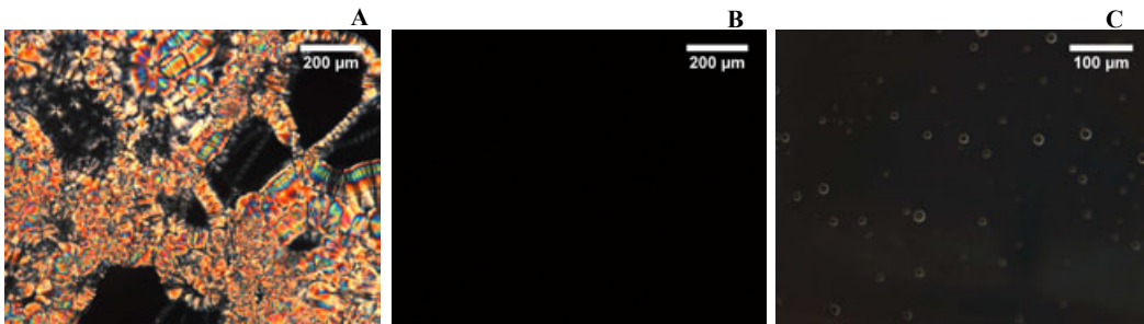
FIGURE 3.19: Polarizing optical microscopy texture of; (A) swollen lamellar phase at H_c=0.4381 , (B) swollen L_x phase at H_c=0.8333 and (C) L_x phase at H_c=1.2829 in the CPC-SHN-Hexanol-Water system at \alpha=2 , \phi_s=30 , T=30^\circ\text{C} .
