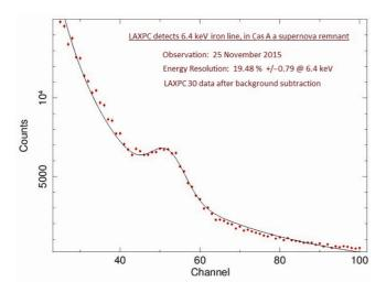
Figure 1. Cas A (supernova remnant) observation of LAXPC30 showing ~20% energy resolution at 6.4 keV.
