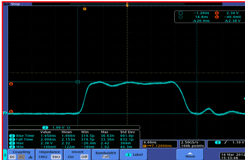
Fig 5.3. Output of SPCM-AQR-14 on oscilloscope
