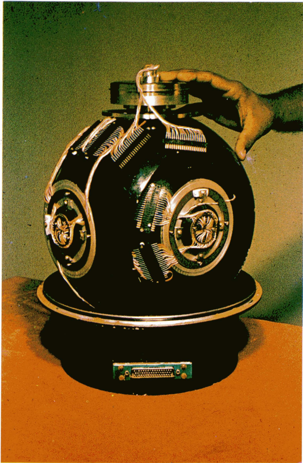
28. SLV-3 Inertial measurement Unit
