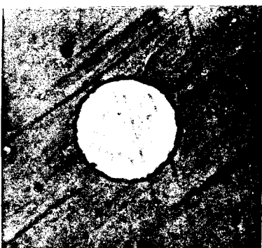
Fig. 4 Organic fibre in polyester matrix developed at NAL (diameter of the fibre 30 \mu m)
