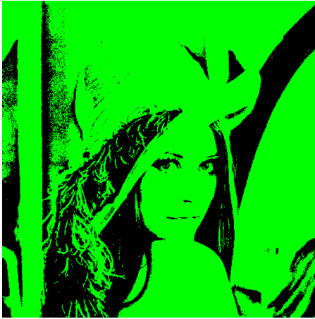
Fig. 15. Image to be displayed during first time interval of pulse width modulation of bit-8 and bit-7 (see right side on Fig. 14) of image Lena.
