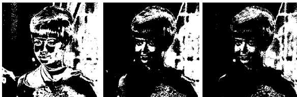
Fig. 10. Bit plane images of bit-7 of primary colors of the image Girl.
