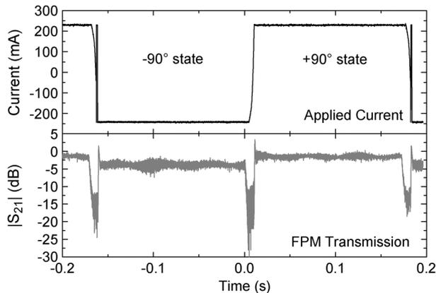
Fig. 5. Applied current: Current modulation pattern provided to the FPM to switch between the nominal  $\pm 90^\circ$  states. FPM Transmission: RF signal at 90 GHz during this modulation.
