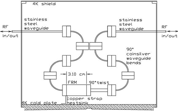
Fig. 2. Waveguide plumbing inside the 4 K dewar shield. Thin-wall stainless steel waveguides (0.03 cm thick) provide thermal isolation between the coin silver waveguides and FPM at 4 K and the dewar shell at 300 K. They are also heat sunk to the dewar's 77 K radiation shield. Thin plastic films act as vacuum windows (not shown).
