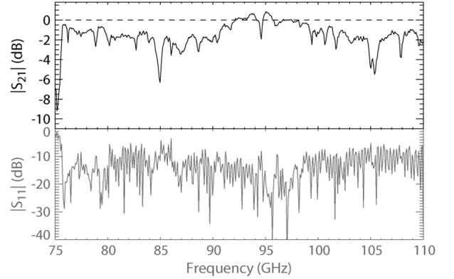
Fig. 3. Average value of  $|S_{21}|$  at the maximum negative current of  $-375$  mA is  $-1.45$  dB. Corrections for the waveguide baseline subtraction are overestimated in the central portion of the band by at least  $0.87$  dB.
