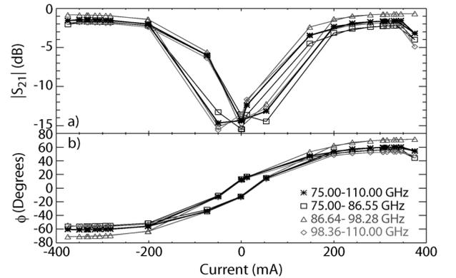
Fig. 4. FPM transmission and phase shift vs. current corrected for losses in the waveguide and ferrite and separated into 3 frequency bins and a full band average. The FPM shows the best transmission above 200 mA of applied current. The phase shift is estimated by applying (2). Over the entire frequency band, the FPM achieves between  $60$  to  $80^\circ$  of rotation.
