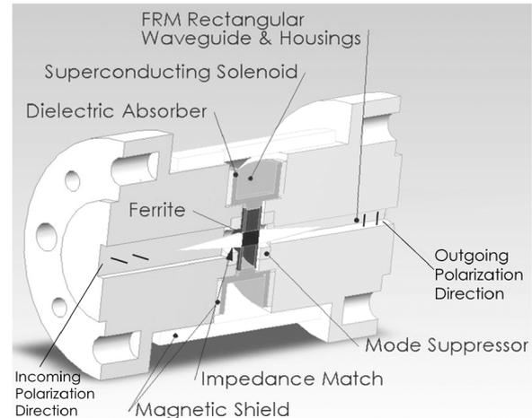
Fig. 1. Cross section of FPM. Alumina tapers impedance match the ferrite to circular waveguide which transitions to rectangular waveguide at the input and output flanges. The rectangular waveguide at the output is rotated  $90^\circ$  with respect to the input waveguide.
