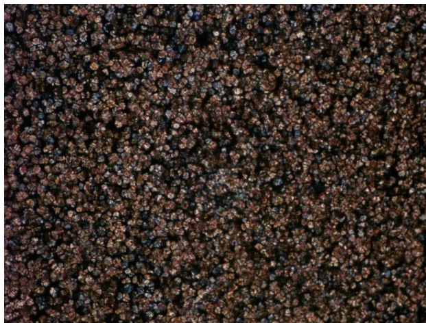
Figure 14: Optical textures for the mesophase of the doped dimer ET14 in 1:1 (dimer: TNF) ratio at 70°C.
