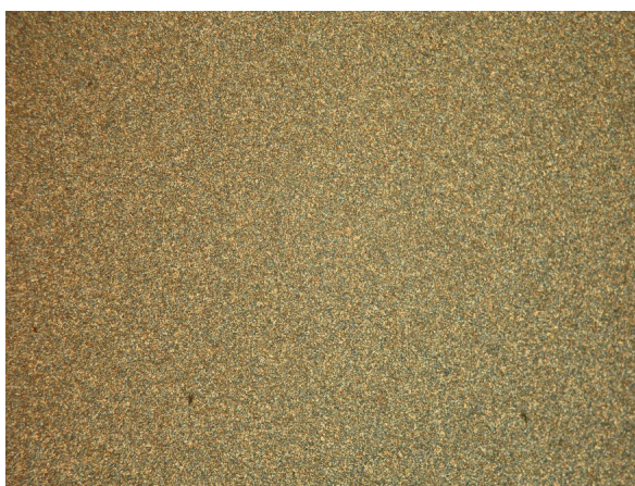
Figure 16. Optical micrograph of 4T8N2BF4 at 76.5 °C on cooling from the isotropic liquid (crossed polarizer, magnification \times 100 ).
