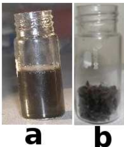
Figure 3.1: A photograph of the dispersions of hexanethiol protected GNPs in a) H1 phase of Triton X-100/water system and b) H2 phase of AOT
