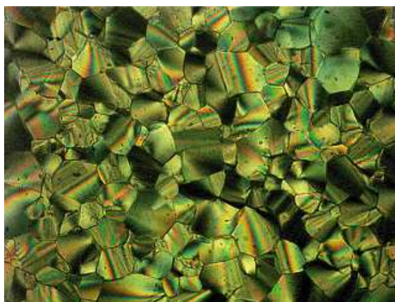
Figure 4.13: Polarising optical micrographic texture obtained for the composite 1 % H AuCl 4 /HAT6 on cooling from the isotropic phase
