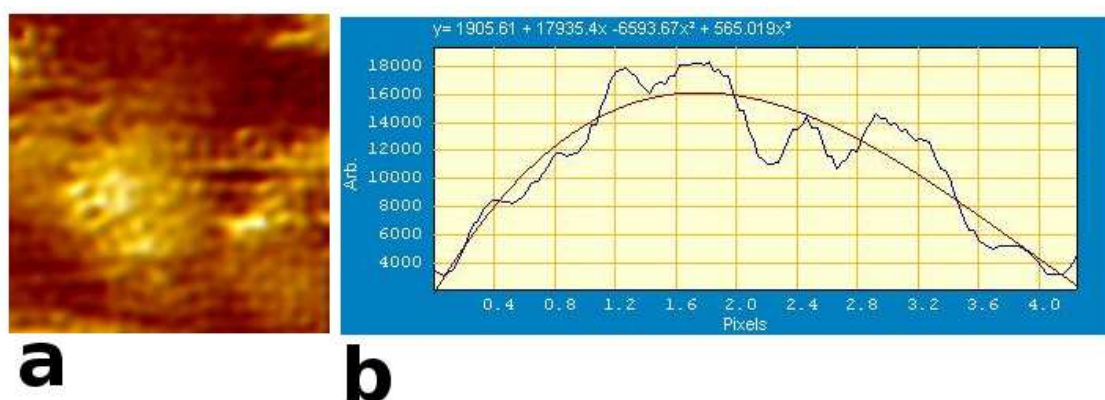
Figure 3.2: a) Scanning tunneling microscopic image of the hexanethiol capped gold nanoparticle and b) line profile for the image
