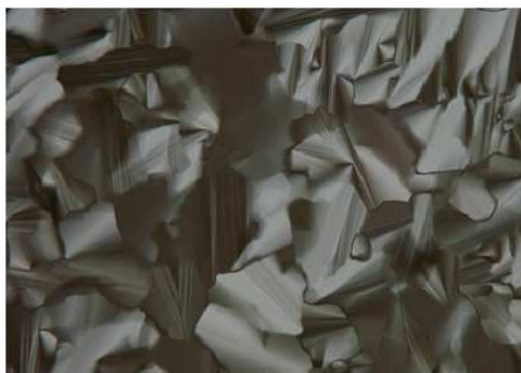
Figure 1.11: Polarising optical micrographic image of the columnar hexagonal phase of Triton X-100/water system
