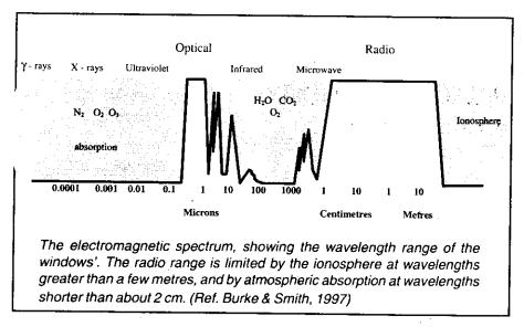
radio waves can pass through the Earth's atmosphere and even through the clouds. Antennas are used to pickup these radio signals. This 100 year-old technique originated from Maxwell and Heinrich Hertz has now evolved to be a very sophisticated technology.
