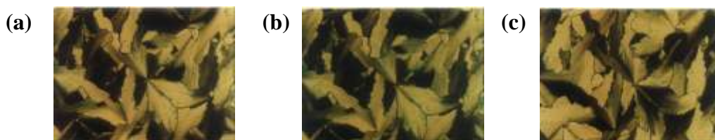
Figure 4.23: Textures of the B_7' phase of compound 4.A.10 obtained under dc electric field, T=128^\circ C . (a) +12 V \mu m^{-1} ; (b) 0V ; (c) -12 V \mu m^{-1} .
