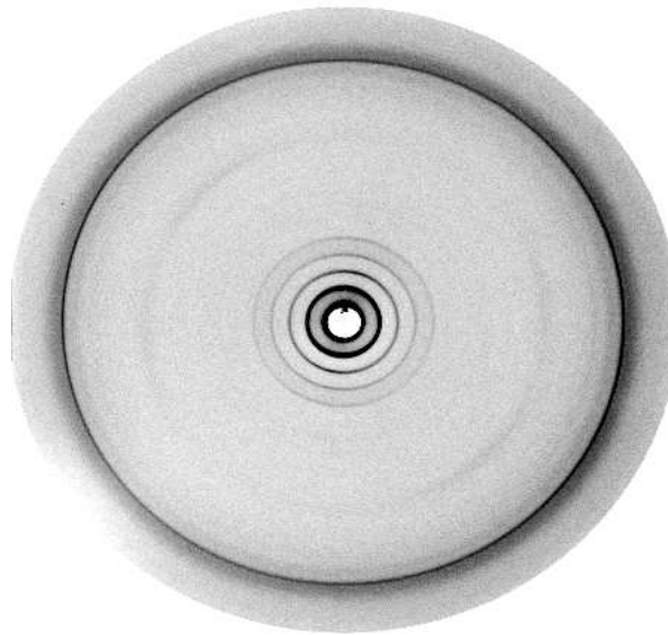
Figure 2.9: Diffraction pattern from an unoriented sample in the gel phase. Concentric rings in the small angle region correspond to the lamellar reflections. Sharp ring in the wide angle region is the reflection from the in-plane hexagonal lattice of the hydrocarbon chains. The diffuse ring at intermediate angles is due to the mylar window of the sample chamber.
