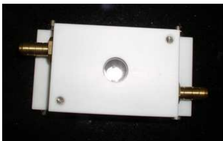
Figure 2.19: A photographs of the chamber used for electroformation.
