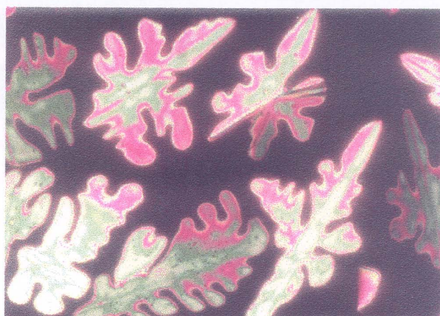
Figure 8.13: An optical photomicrograph obtained for the B_1 phase of compound 8.B.1 on cooling the isotropic phase.
