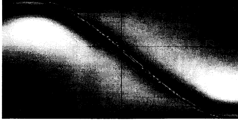
Figure 3.13 : Simulated texture of half a pitch of the chiral domain. Only quarter pitch was simulated at a time for computational convenience. The vertical line is due to this reason.
