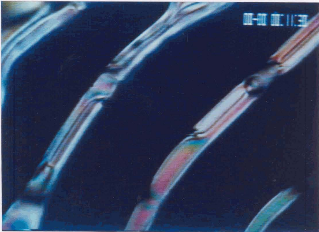
Figure 6.13: Sequence of photographs taken between crossed polarisers during fast heating. The isotropic phase forms channels which are roughly parallel to the stripes.
