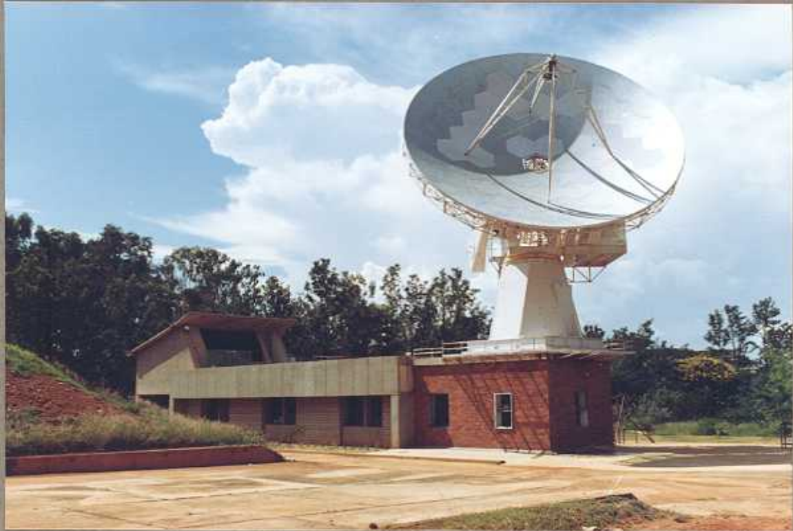
Figure 3.1 (a): The 10.4-meter millimeter-wave radio telescope at the Raman Research Institute campus, Bangalore.
