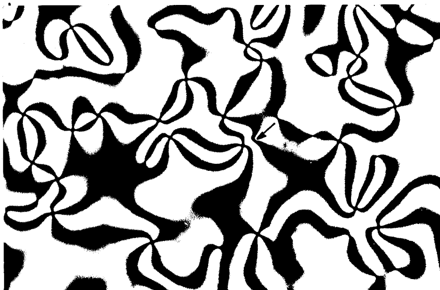
Figure 6.11b. Same area of the sample as in Fig. 6.11a at 38.7^{\circ}\text{C} . Note that the +3/2 defect has split into a +1 and a +1/2 defect (x 920).
