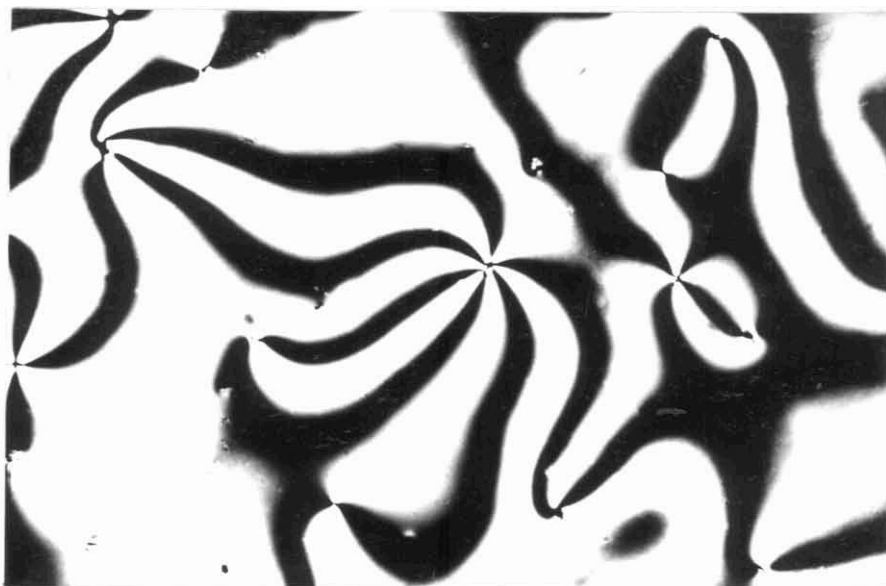
Figure 6.6. A relatively isolated +3/2 defect in Mixture II at 53.2^{\circ}\text{C} , crossed linear polarisers (x 1920).
