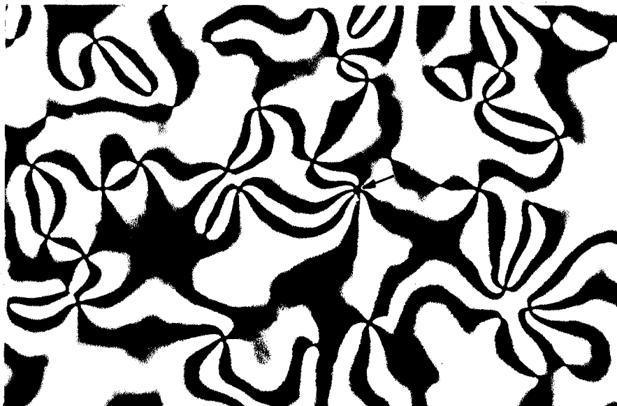
Figure 6.11a. A +3/2 defect (indicated by an arrow) in Mixture I at 36.2^{\circ}\text{C} , crossed linear polarisers (x 920).
