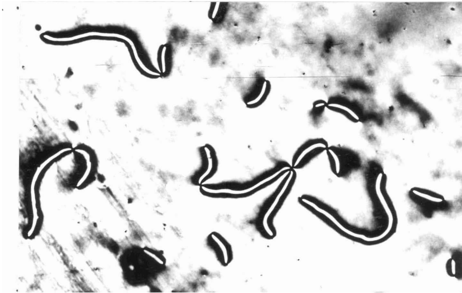
Figure 6.9. An inversion wall of the first kind with a -3/2 disclination, in Mixture I at 28^{\circ}\text{C} , crossed linear polarisers (x500).
