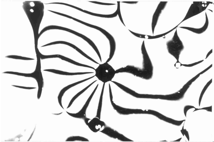
Figure 6.10. 12 brushes around an isotropic droplet in Mixture III at 57^{\circ}\text{C} , crossed linear polarisers (x857).
