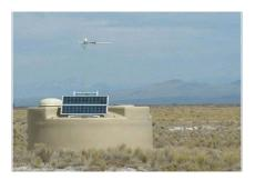
Figure 4. A water tank detector in the Pierre Auger observatory in Argentina.
