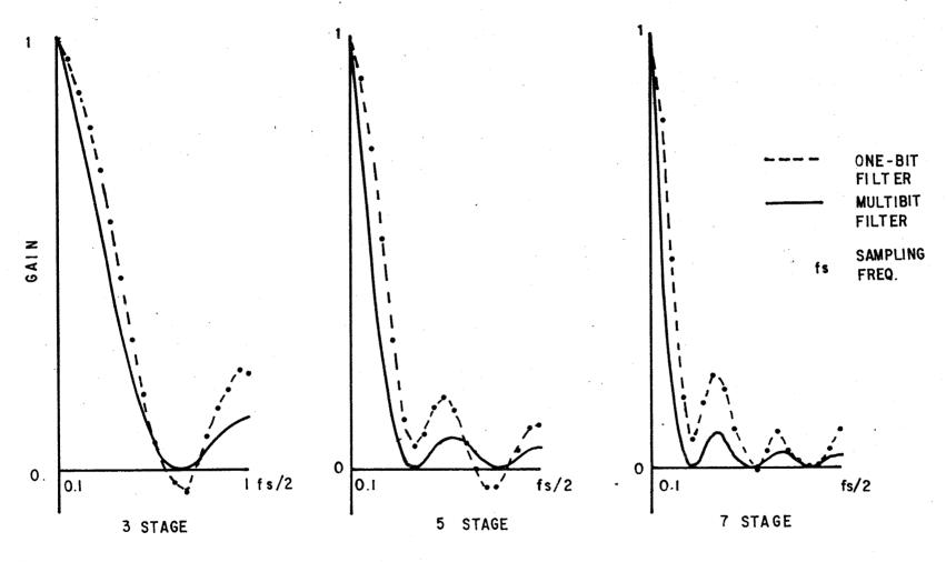
FIG.A.5 FREQUENCY RESPONSE OF MULTIBIT & ONE-BIT DIGITAL FILTERS
