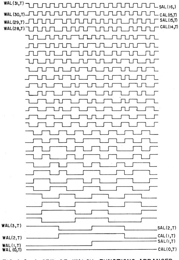
FIG. A.2 A SET OF WALSH FUNCTIONS ARRANGED IN SEQUENCY ORDER. (BEAUCHAMP-1984).  $f(t) = a_0 \text{ WAL } (0,t) + \Sigma a_n \text{ WAL } (n,t)$  $a_n = \frac{1}{T} \int_0^T f(t) \text{ WAL } (n,t) dt.$
