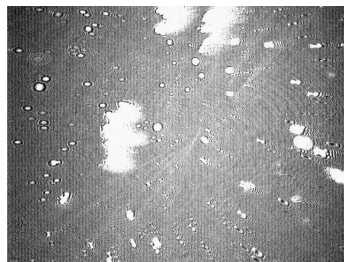
Figure 2.17: Brewster angle microscopy image of cholesteryl myristate. Figure shows the presence of bright irregular shaped 3D crystallites occurring at an A/M of 391 \text{ \AA}^2 .
