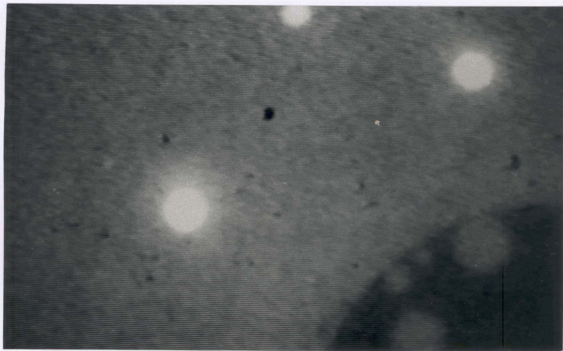
Figure 2.9 Fluorescence image of 8CB monolayer at 25^{\circ}\text{C} 18\text{\AA}^2 A_m showing co-existence of LE (black), D_1 (grey) and D_2 (bright) domains. Scale of the image: 1080\mu\text{m} \times 750\mu\text{m} .
