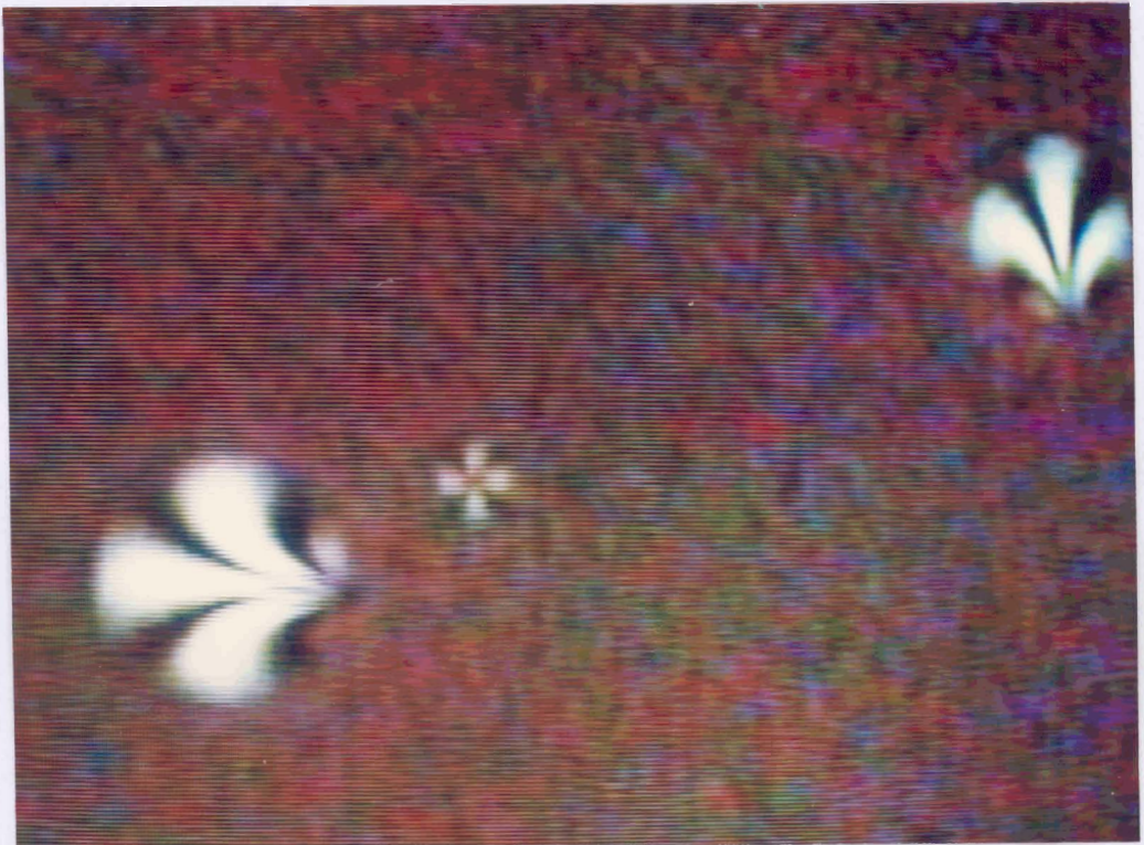
Figure 2.16 Image of D_3 domains at 30^\circ\text{C} under a polarising microscope. (a) Two domains exhibiting a boojum texture. (b) Two domains exhibiting boojum texture and one with ordinary schlieren texture. Scale of the images: 400\mu\text{m} \times 300\mu\text{m} .
