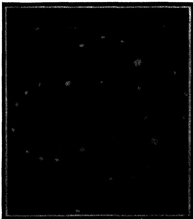
Figure 5. Dynamic reflections by sodium nitrate at 225° C (after Raman and Nilakantan, May 1940).
