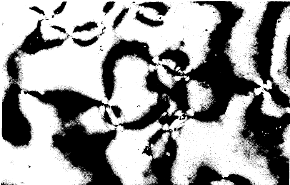
Figure 2. Disclinations of strength \pm 1/2 and \pm 1 seen in a room temperature nematic mixture. Crossed linear polarizers and illumination with sodium light ( \times 600 ). The dark rings around disclinations of strength \pm 1 are due to the collapse of the director in the third dimension.
