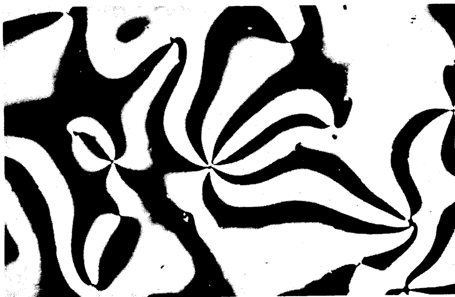
Figure 4. A +3/2 defect in a mixture of 20 wt% leucoquinizarin with octyloxycyanobiphenyl. Illumination with white light ( \times 600 ).
