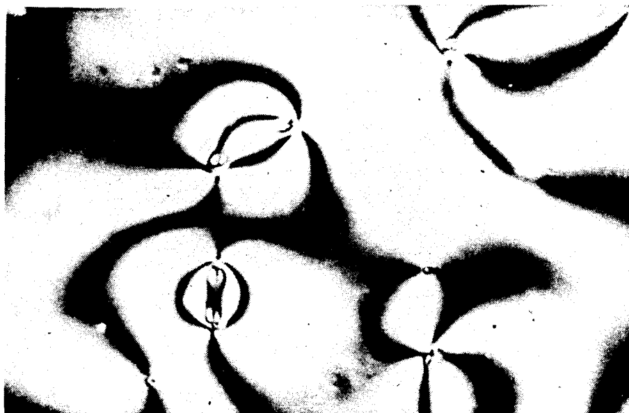
Figure 5. A \pm 3/2 pair of disclinations in a mixture of 12 wt% leucoquinizarin and p -cyanophenyl- p - n -heptylbenzoate ( \times 650 ).
