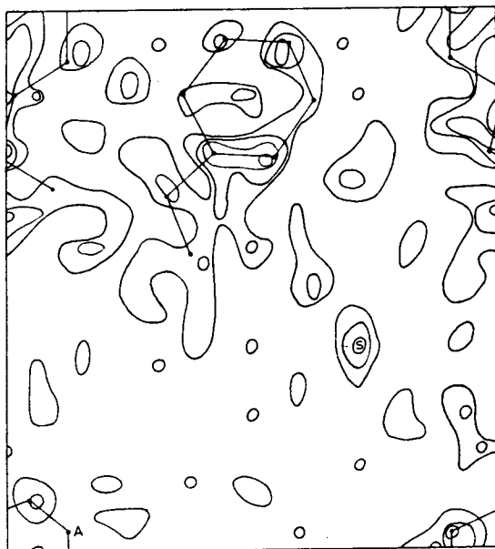
Figure 7. The true structure consists of 2 molecules, of 8 equal atoms each, with the orientations and relative spacings shown. The MEM map obtained by refining random starting phases reveals most of the structure except the absent atom A . There is one strong spurious peak S .
