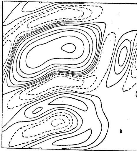
Figure 6. The dirty map made with the Fourier coefficients \rho_{mn} of the model in Fig. 4 ( |m|, |n| \leq 3 ). This is the convolution of Fig. 4 with Fig. 5.
