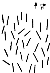
Figure 1. Schematic diagram of the arrangement of rod-like molecules in the orientationally ordered nematic liquid crystals. \vec{n} is the direction of average orientation of the molecules.
