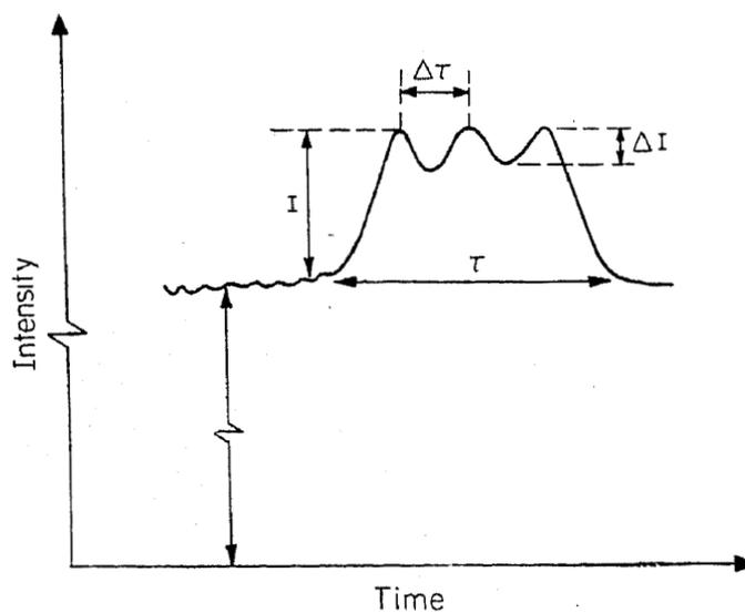
Figure 2. Explanation of the burst parameters.
