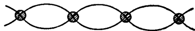
Figure 4 A qualitative picture of the Borrmann effect in x-rays. The nodes of the standing wave coincide with the atomic positions giving minimum absorption.
