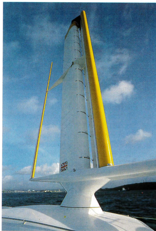
Figure 26. The bearing on which the whole airplane part is completely free to rotate. The flap on the wingsail is in the operating position.
