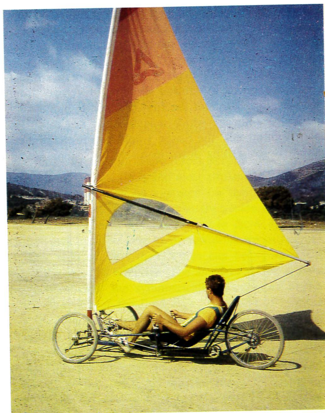
Figure 12. A land yacht on three bicycle wheels. The front two are used for steering and the sail is that of a windsurfer.
