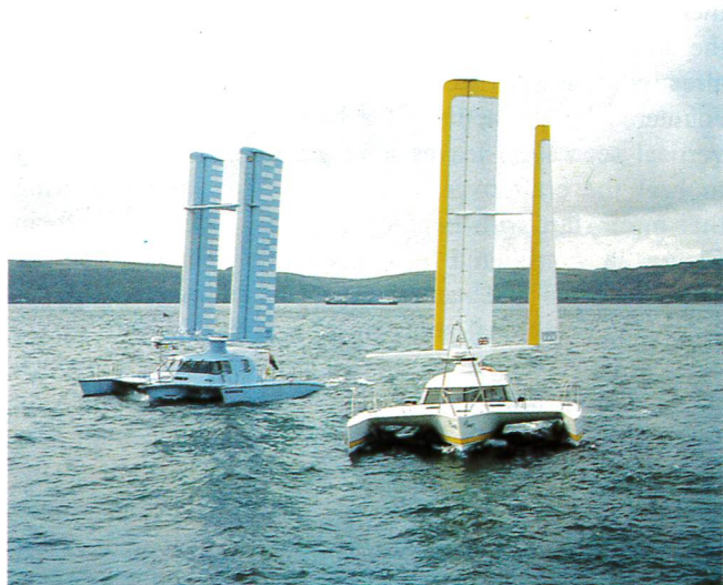
Figure 24. Blue Nova to the left was the first wing powered boat to cross the Atlantic and back, and went safely through a severe hurricane in the process. To the right is Zefyr , the latest monoplane version of the Walker Wingsail. The tail is clearly seen on this boat but is partly hidden from view in the other.
