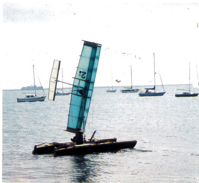
Figure 22. A catamaran with a true wingsail. It is an asymmetric one, and so has to be flipped over the top to sail on the other tack. The white tail at the back functions like an airplane elevator, and is set to control the angle to the wind of the main wing.
