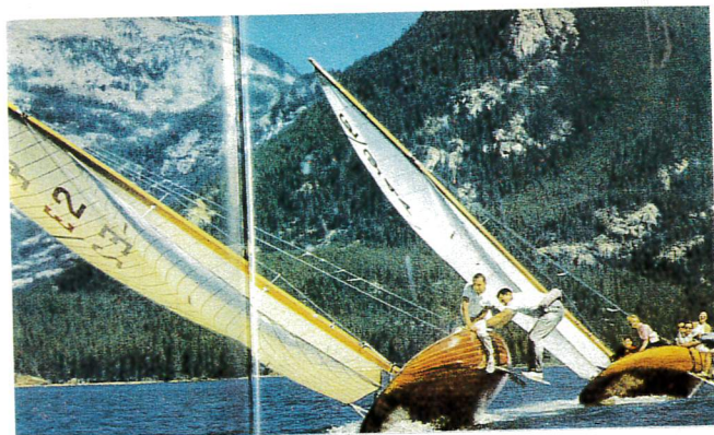
Figure 28. Countering the heeling moment when going to windward with agile human balast. Weekend sailors tend to consider the discomfort associated with this angle of heel a thrilling bonus not to be missed.
