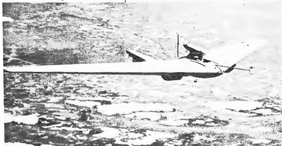
The plywood N9M, a one-third scale model, successfully simulated the XB-35 control and stability characteristics.
