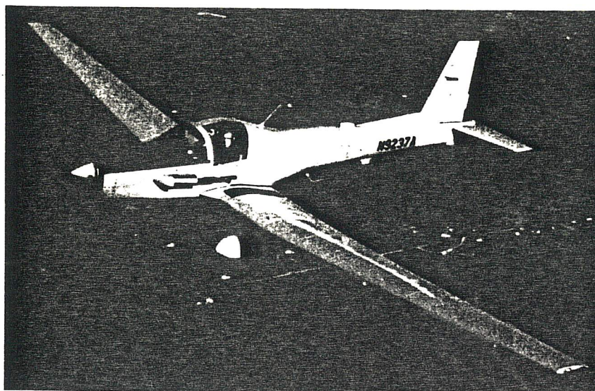
Left Schweizer Aircraft is promoting its 2-37A light surveillance aircraft fitted with the Hughes AN/AAQ-16 forward-looking infrared night vision system. Below The system's sensor is mounted in a turret below the fuselage on the centreline just forward of the wing trailing edge
