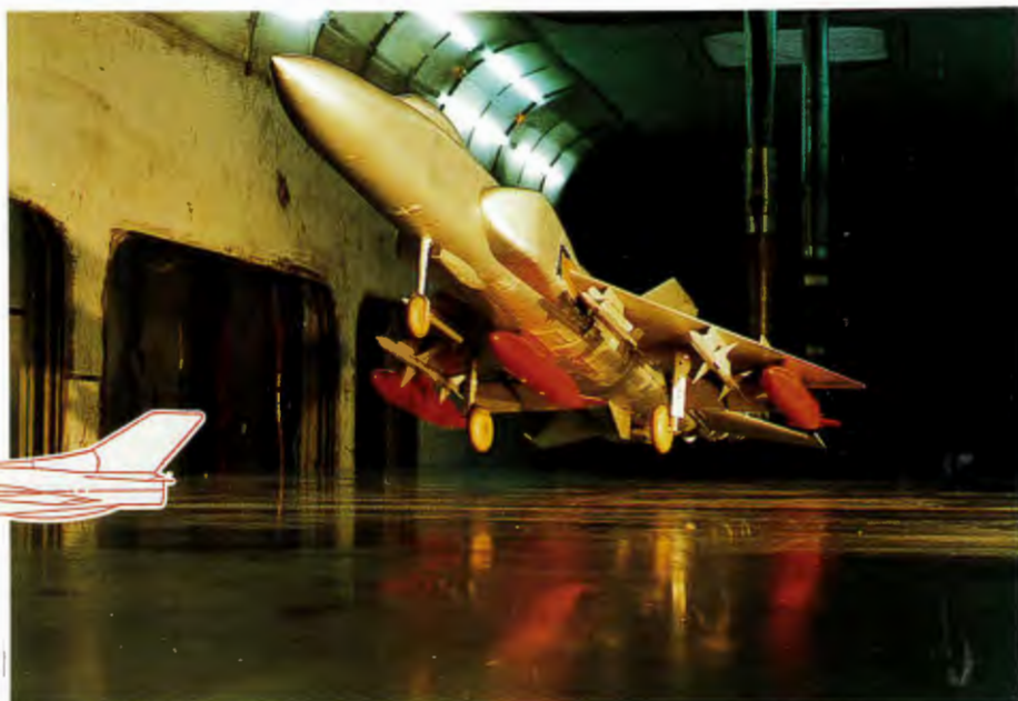
飛機起飛着陸模擬試驗 Aircraft testing with a Ground Plane
