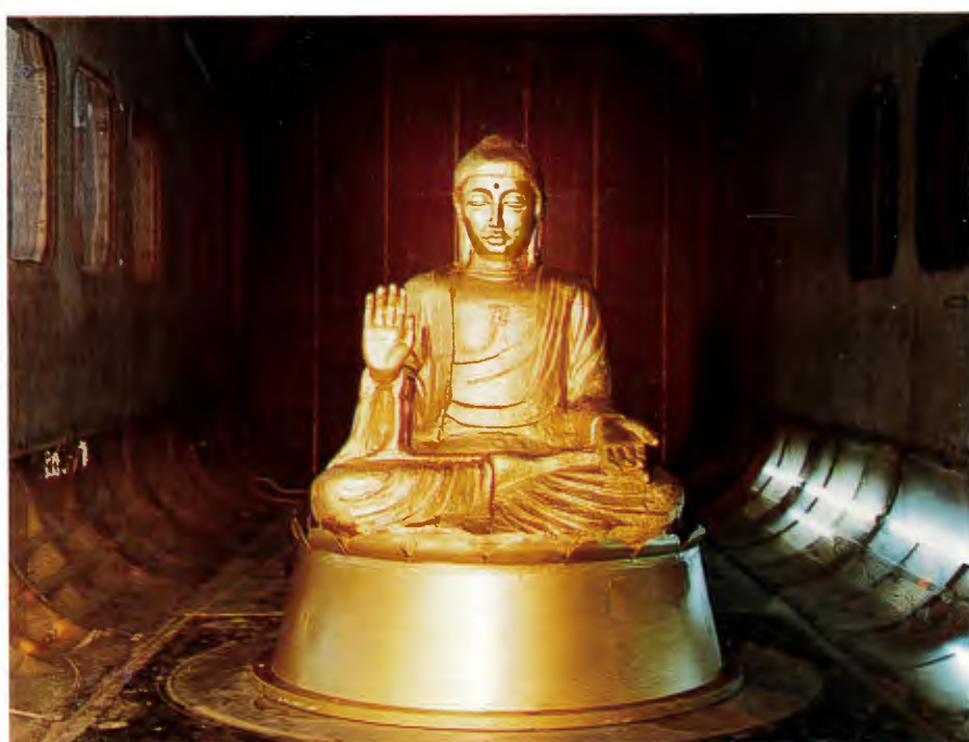
香港天壇大佛的風載試驗 Wind load testing for large buddha statue
