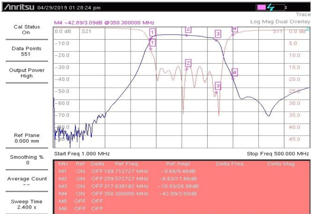
Figure 18. Measured S21, S11 Response of the Microstrip Band-pass filter
