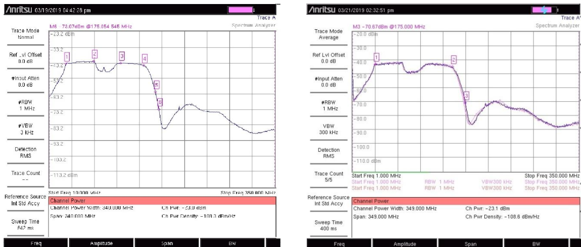
Figure 21a. RF power spectrum of the first sub-band from 40MHz – 175MHz
