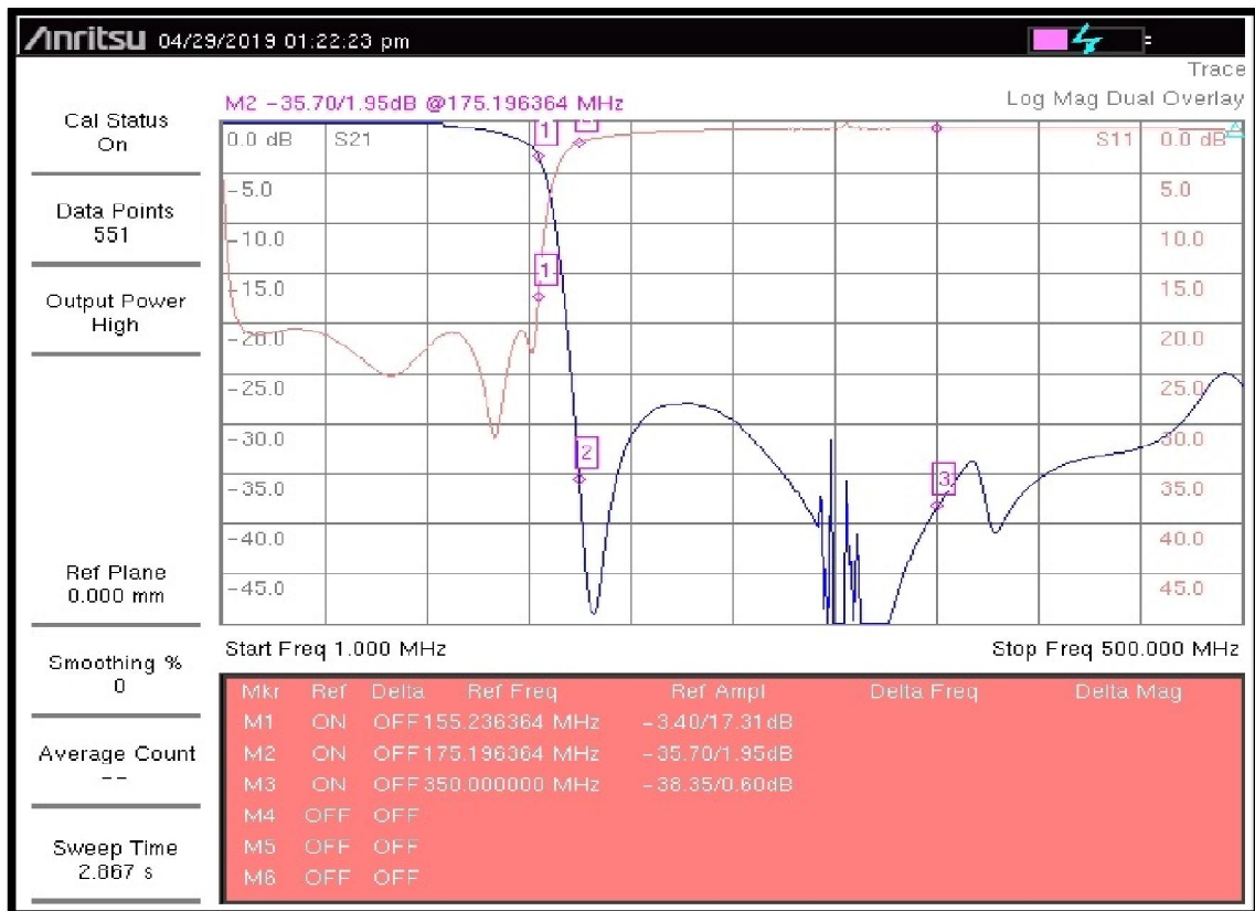
Figure 13. Measured S21 and S11 Response plot of the microstrip low-pass filter
