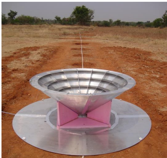
Fig. 10. Front view of the prototype discone antenna placed over a metallic reflector using electromagnetically transparent pink Styrofoam.
