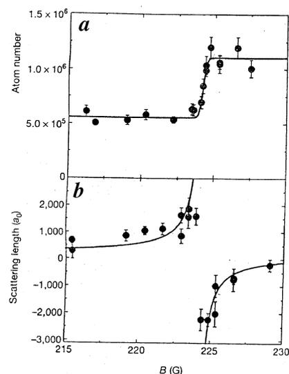
**Figure 4.** *a*, Atom loss as the magnetic field is ramped across Feshbach resonance in  $^{40}\text{K}$  (Reprinted with permission from ref. 11 *Nature*). *b*, Previous measurement of Feshbach resonance.
