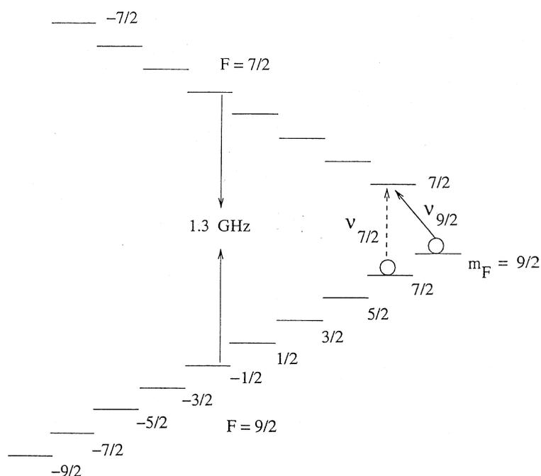
**Figure 1.** Zeeman sub-levels of the hyperfine structure of  $^{40}\text{K}$  ground states,  $F = 9/2$  and  $F = 7/2$  (reprinted with permission from ref. 5 (2003) AAAS).
