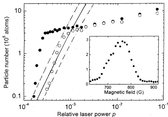
**Figure 5.** Number of trapped particles as a function of  $p = (I/I_0)$ , relative intensity of the laser on both sides of Feshbach resonance. Open circles are for  $B = 1176$  G and  $a = -3500 a_0$ . Closed circles are for  $B = 764$  G and  $a = +3500 a_0$ . (Inset) Optimum magnetic field for production of dimers (Reprinted with permission from ref. 13 (2003) AAAS).
