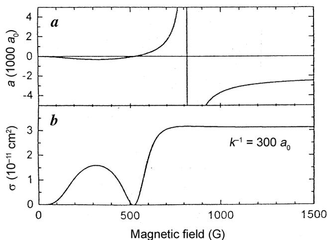
**Figure 3.** **a**, Model curve approximating theoretical calculations of s-wave scattering length for  $^6\text{Li}$  atoms in the two lowest spin states against the magnetic field. **b**, Corresponding behaviour of scattering cross-section (from ref. 8).
