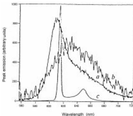
**Figure 3.** The emission spectrum of a  $\text{TiO}_2$ -rhodamine system at three different pump powers. Curve *b* has been scaled up by a factor 10, while curve *c* has been scaled down by a factor of 20. Pump power for *b* < pump power for *a* < pump power for *c* (figure from ref. [17]).
