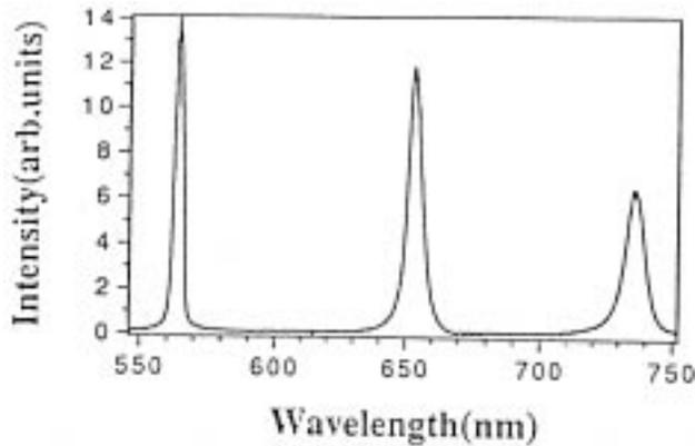
**Figure 9.** Laser emission from a three-layer stack (from ref. [29]).
