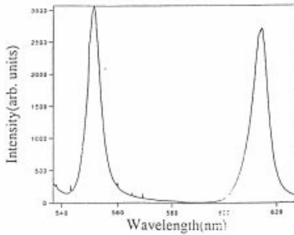
**Figure 7.** Emission from a braided pair of nylon fibers, one with pyromethene dye and the other rhodamine. Both contain  $\text{TiO}_2$  scatterers (from ref. [28]).
