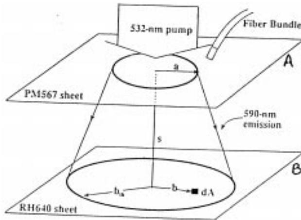
**Figure 8.** The polymer sheets A and B both contain  $\text{TiO}_2$  scatterers, but different dyes. Sheet A is pumped with an external laser at 532 nm, while its emission pumps sheet B. The emission of both sheets can be viewed using the fiber bundle at the top (from ref. [29]).
