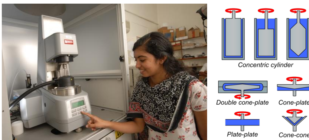
Figure 4: (Left) An Anton Paar stress-controlled MCR 501 rheometer in the author's lab. In this picture, the rheometer is being operated by an ex-member of our laboratory, Dr. Paroor Harsha Mohan. (Right): Pictures of some commonly used rheometer geometries. Samples (shown in blue) are loaded in the geometry (usually made of stainless steel and depicted in grey). Oscillatory and rotational strains/ stresses are applied on the sample by the geometry and the stress/ strain responses are measured using a motor-transducer assembly.
